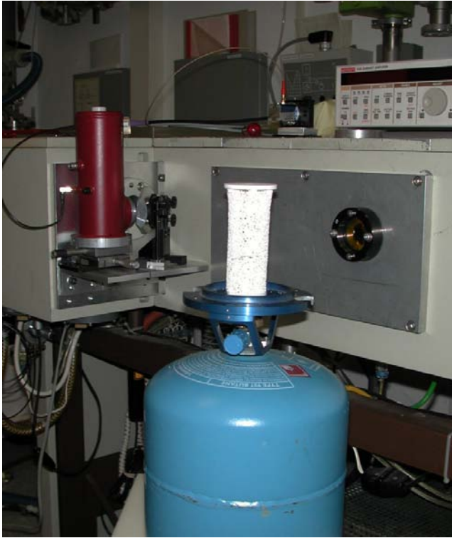
Figure 10.8. Spectroscopic set-up for the FTIR measurement of the foam ceramic emitter spectrum.
