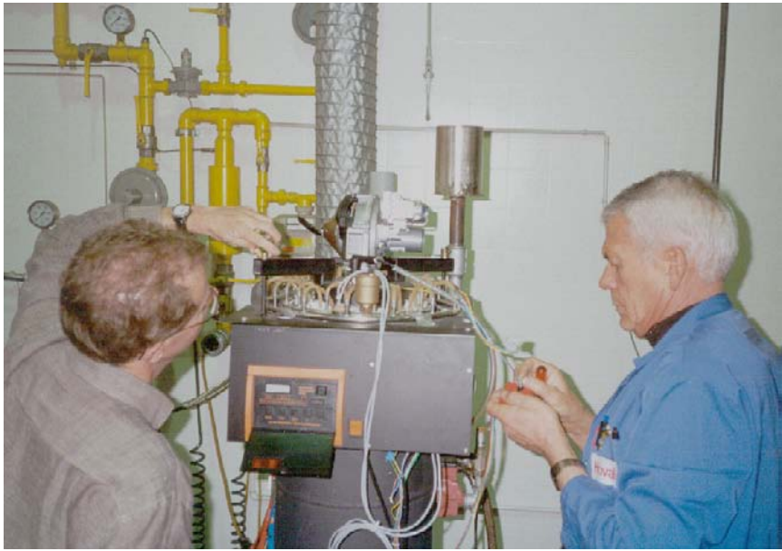
Figure 10.5. The photograph shows the Hoval TPV prototype heating system in preparation for a long-term test.
