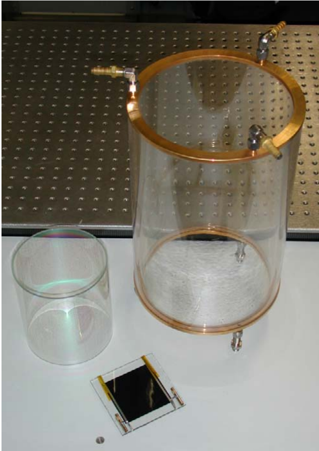
Figure 10.13. Photograph of some components, which can be used in a modified way in a future thin-film TPV system: water filter, SnO 2 filter tube and CIGS solar cell.
